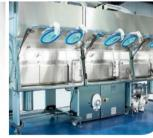
Extract Technology's Cell Therapy Isolators are designed to provide an ergonomic and practical alternative to traditional clean rooms for stringent cGMP and international regulations for the production of cells for clinical use.
