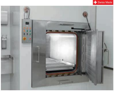
Double door chamber forms a barrier between hot and cold zones
