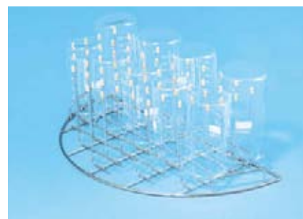
Universal carrier, art. no. 440 085 with pins for holding glassware and utensils, ø 570 mm, h 183 mm, 2–3 carriers per level
